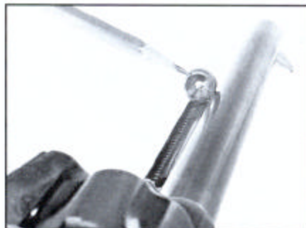
Bullseye-style ejector rod head is correct for 1878-manufacture M1873.
